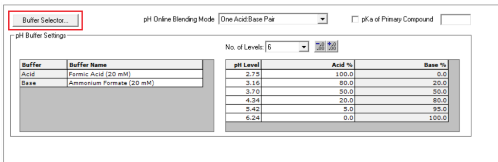
Figure 5. Online Preparation of pH for a broad Chemistry System Screening Study
